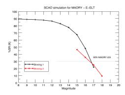
Fig. 3. SCAO Strehl ratio vs. R magnitude.
