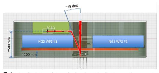
**Fig. 1.** MAORY NGS WFS module layout. Three low-order and Truth WFSs lie on top of a counter-rotating plate, while a SCAO WFS is on top.
